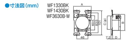
Table with dimensions A, B, C(φ), D for products WF1330BK-WK, WF1430BK-WK, WF3630B-W.
